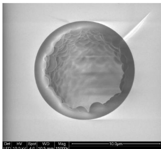
Scanning electron micrograph of the end section of a 10  $\mu\text{m}$  inner diameter polystyrene-divinylbenzene porous layer open tubular (PLOT) column made at the Department of Chemistry and intended used for peptide and protein separations for identification of cancer stem cell markers.
